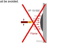
Irrespective whether the VP 10-500 has been applied to cold or warm metal, the metal temperature must not exceed approx. 130-150 °C up to the start of the curing process. If there is no suitable temperature measuring device available, we recommend the use of the self adhesive temperature indicators, which can be ordered at MultiMetall.
