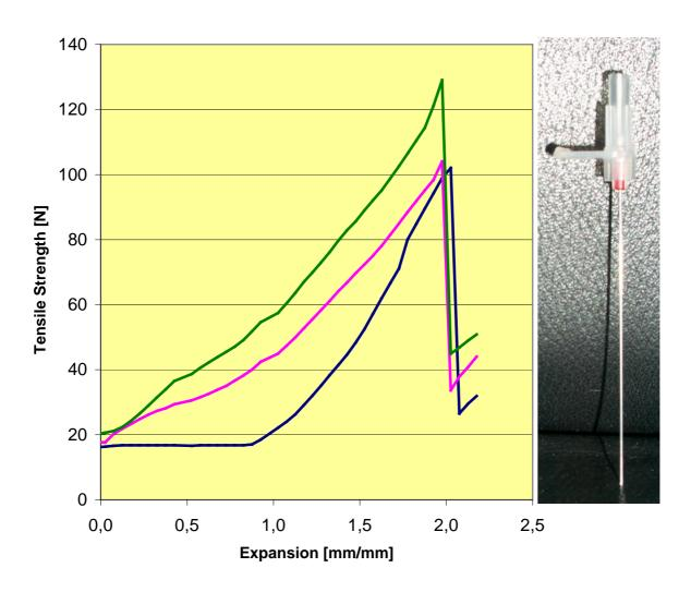
The above figure shows typical values to pull needles (steel) out of a hub (polypropylene) after bonding with Byllux 5791.
