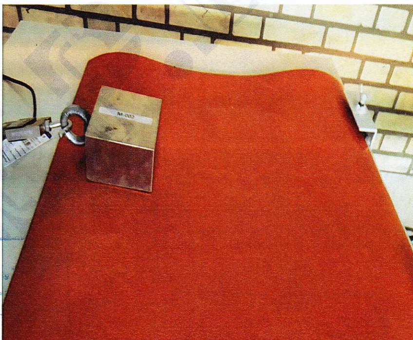
Figure 2: EUT under The Slip resistance Test
